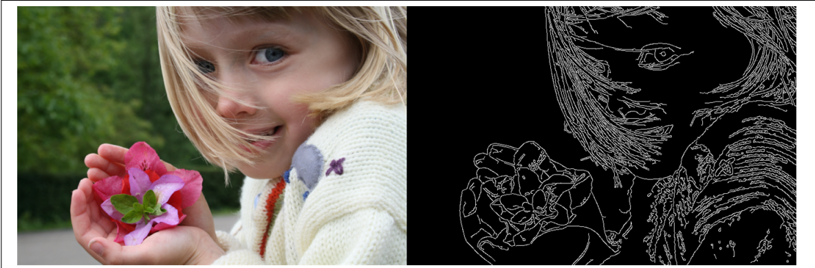
Figure 4.25: Example of edge detection. Taken from http://en.wikipedia.org/wiki/File:EdgeDetectionMathematica.png
