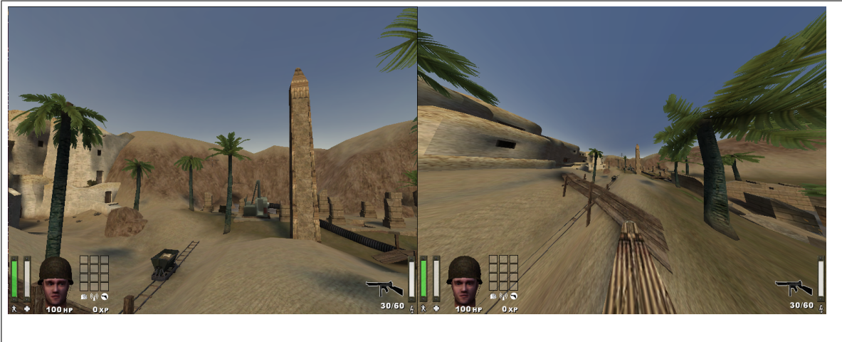
Figure 4.38: The left is the image when the FOV is selected to be a minimum, the right is the maximum. The player position has not changed!
