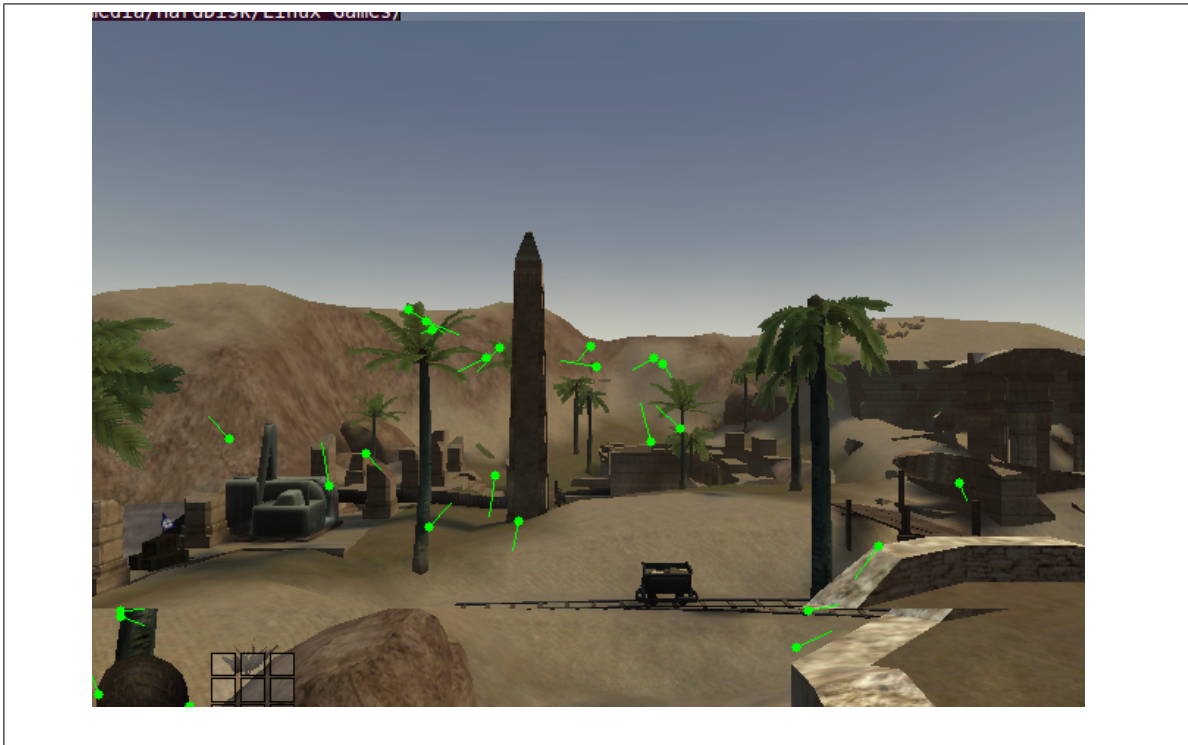
Figure 4.44: Fast panning - most Harris points are lost and the ones that remain are anomalous
