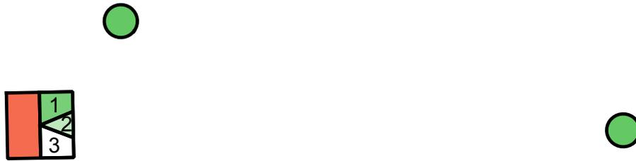
Figure 2.5: Example of a robot having three distance sensors to probe food items: sensor 1 is the left food item sensor, 2 the middle one and 3 the right one. The higher the measured value of the sensor is, the darker the green fill color is. Inactive sensors are white. Poison sensors are not represented.
