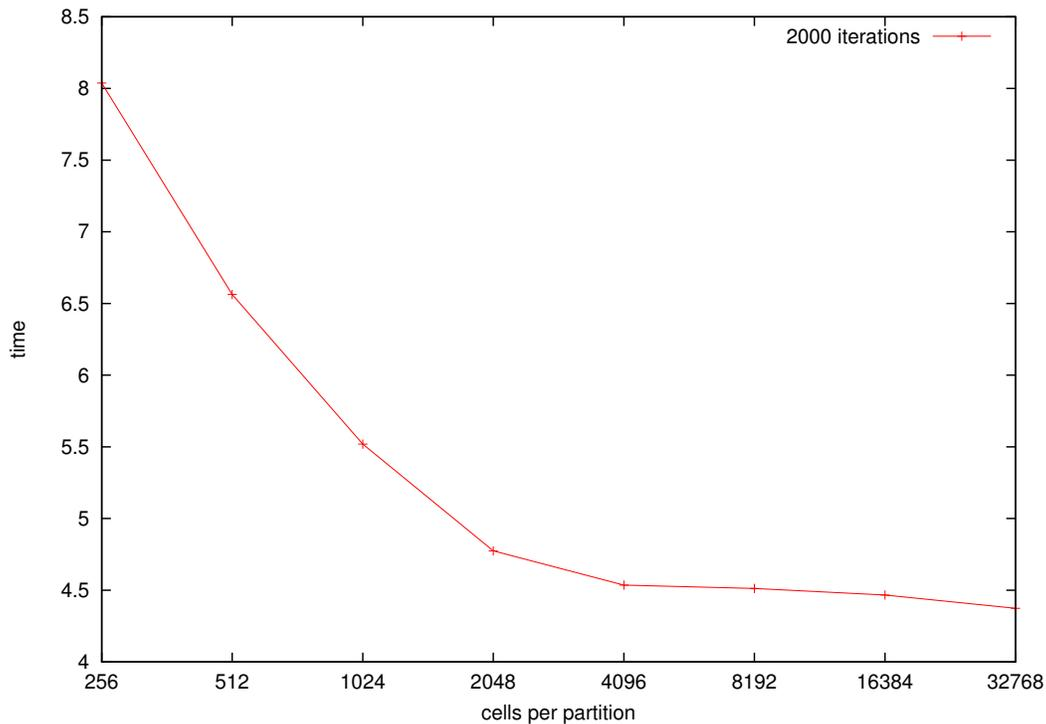
Figure 3.11: Plot of estimated execution time for 2000 iterations of `res_calc` against the number of cells per partition. Note that the horizontal axis is on a log-2 scale. The design has 8 pipelines and runs at 240MHz. Note how for values of  $C_{pp}$  less than 2048 the execution time rises very steeply. This is when the proportion of halo data to non-halo data becomes too large and the PCIe transfers dominate and become a bottleneck.
