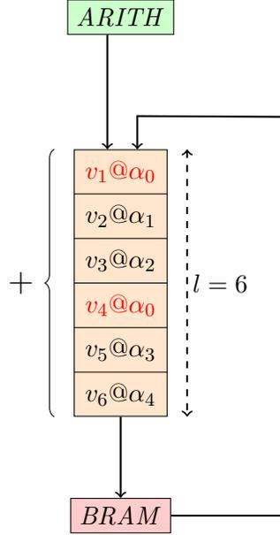
Figure 4.1: Architecture diagram of the accumulation part of the accelerator design showing the conflicting values of  $res$  being computed in the accumulator pipeline. The conflicting values for address  $\alpha_0$  are shown in red.
