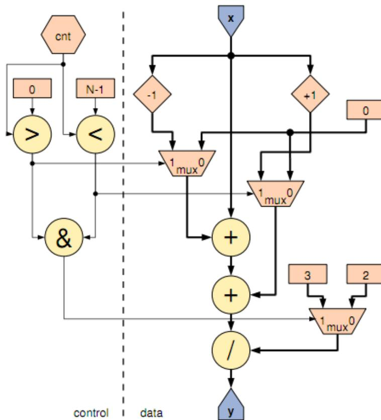
Figure 2.6: The dataflow graph resulting from the code in Listing 3. Note: the *stream.offset(x, -1)* and *stream.offset(x, +1)* expressions are shown here using the rhombuses with +1 and -1, evaluating the value of *x* one cycle in the 'future' and one cycle in the past respectively. The other nodes have the obvious meanings.
