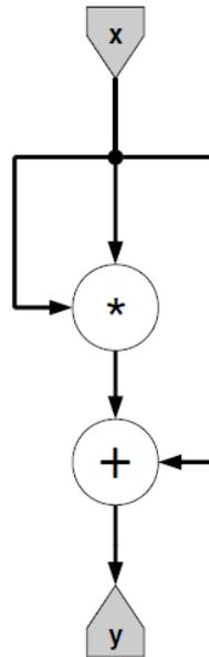
Figure 1.2: A simple dataflow graph that implements the function  $y(x) = x^2 + x$ . The adder and the multiplication nodes are fully pipelined, enabling a throughput of one result per cycle, thus providing us with the intuition for accelerating floating point calculations
