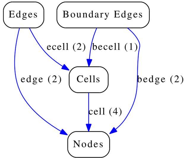
Figure 2.4: Diagram showing the maps between the mesh elements. The dimension of the map is shown in parentheses next to the name. Thus the map *edge* relating edges to nodes with dimension 2 means that for each edge, there are two nodes associated with it.
