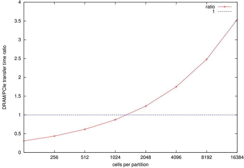
Figure 3.12: Plot of estimated DRAM to PCIe transfer time ratio ( $\frac{t_{DRAM}}{t_{PCIe}}$ ) against the number of cells per partition. Note that the horizontal axis is on a log-2 scale. The design has 8 pipelines and runs at 240MHz. Notice that for values of  $C_{pp}$  less than 2048 the ratio of DRAM to PCIe transfer time drops below one and the whole design is dominated by halo transfers, greatly decreasing DRAM bandwidth utilisation.
