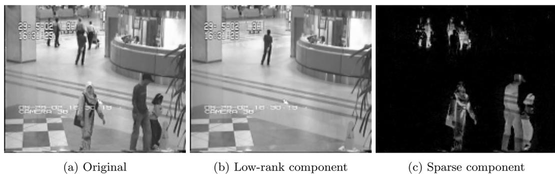
Figure 1.4: Example of background subtraction from a surveillance video. A single video frame is shown. The low-rank component (b) contains the background and the sparse component (c) contains the foreground. The man in (b) was not moving and hence was incorporated in the background. Image taken from [18].
