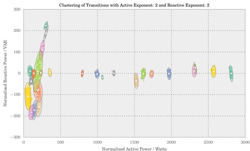
(a) Complex power plane in author's home. In this plot, the sensor offset has been corrected for ease of comparison with 7.1b.
