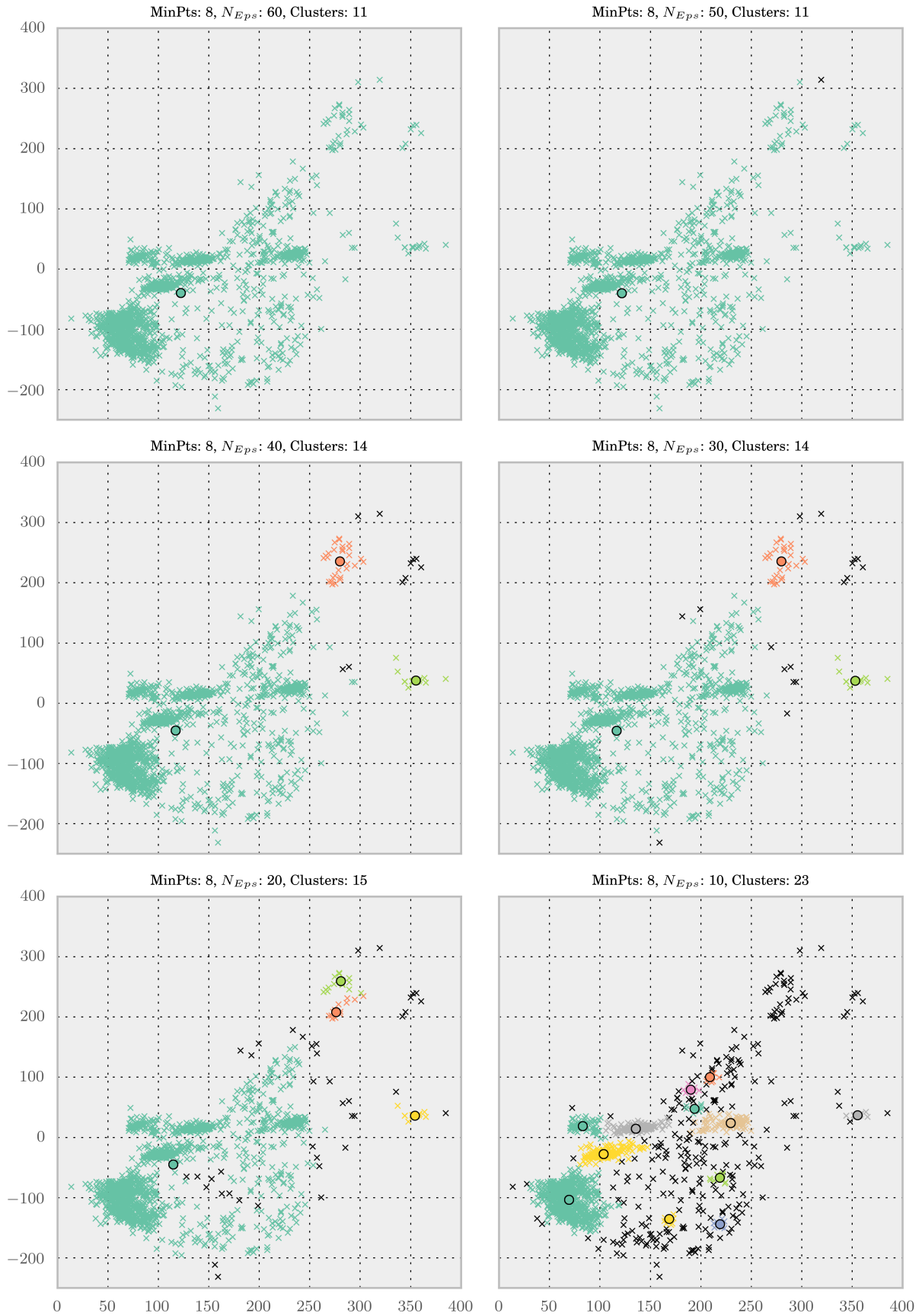
Figure 4.11: Visualising the outcome of DBSCAN for decreasing N_{Eps} values for < 400\text{W} active power. Black circles represent centroids, whilst \times 's are individual samples. The samples are colour-coded to the centroid. Black \times 's are points classified as Noise by the algorithm.
