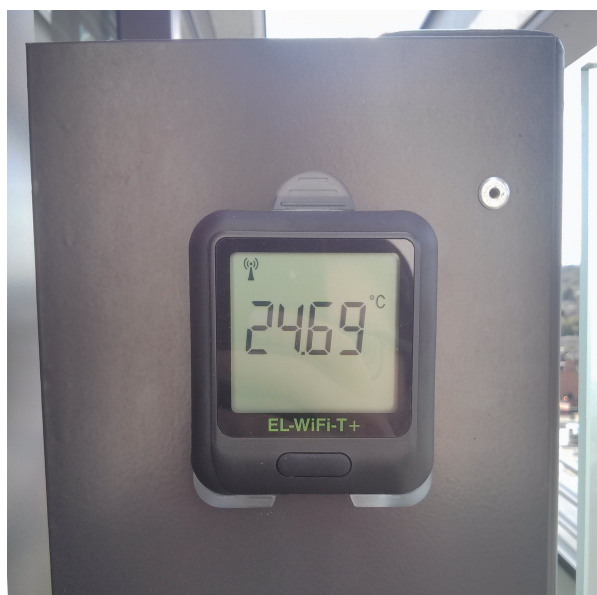
Figure 2.1: Externally mounted temperature sensor
