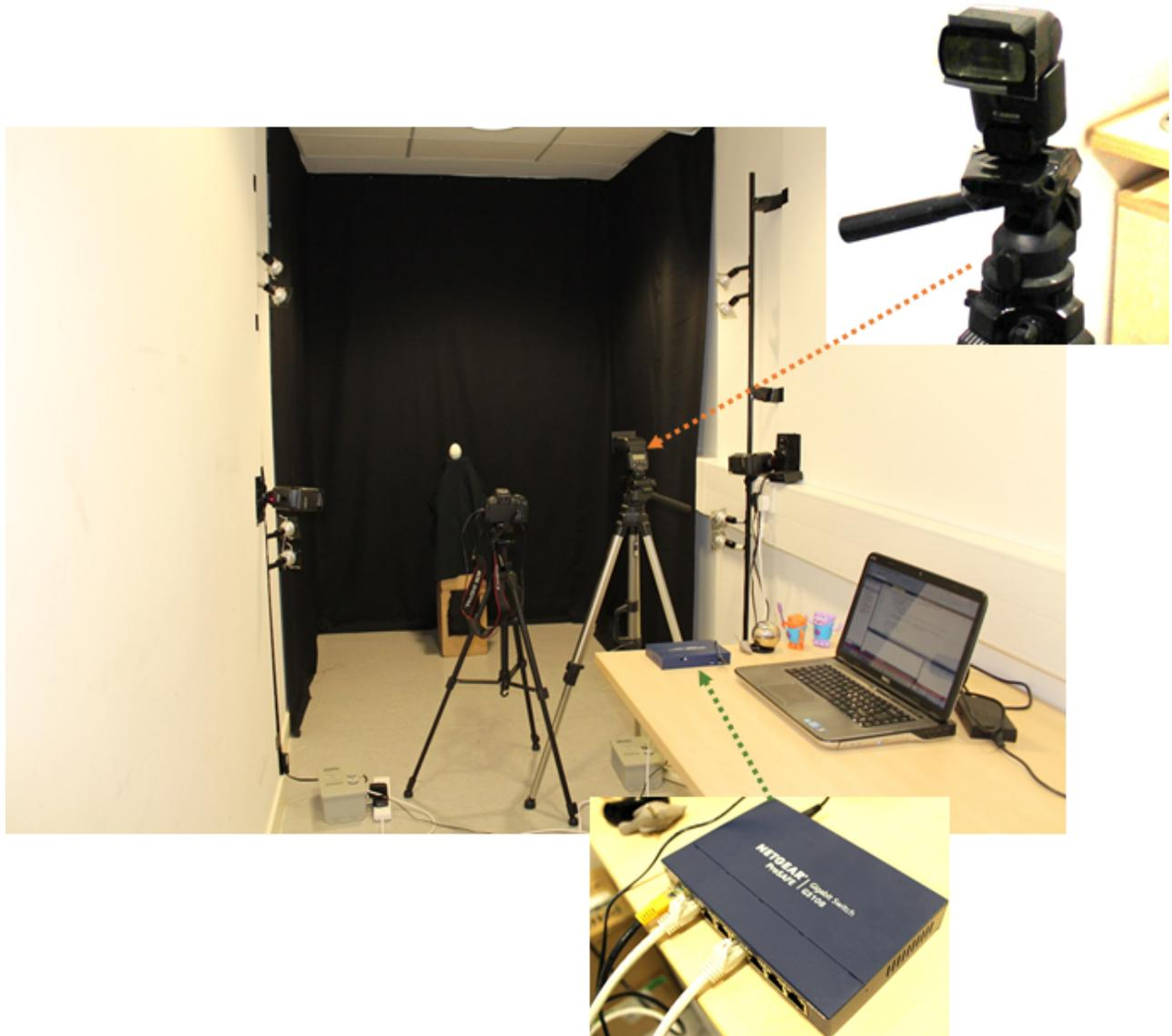
Figure 3.1: Self built Reflectance acquisition setups with DSLR and Speedlite flashes
