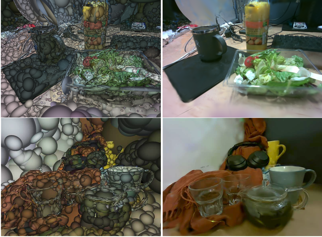
Figure 4.6: Self-captured Scenes: Challenging scenes and objects, for example, transparent glasses and the crinkled texture of salad, are captured by our monocular SLAM running live.
