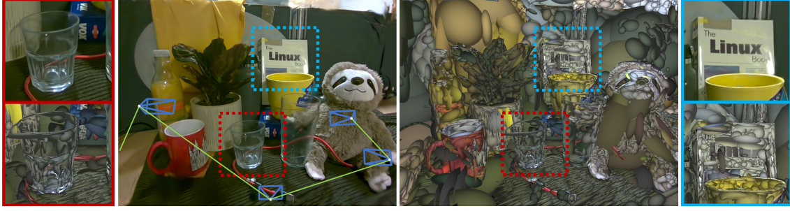
Figure 4.1: From a single monocular camera, we reconstruct a high-fidelity 3D scene live at 3 FPS. For every incoming RGB frame, 3D Gaussians are incrementally formed and optimised together with the camera poses. We show both the rasterised Gaussians (left) and Gaussians shaded to highlight the geometry (right). Notice the details and the complex material properties ( e.g. transparency) captured. Thin structures such as wires are accurately represented by numerous small, elongated Gaussians, and transparent objects are effectively represented by placing the Gaussians along the rim. Our system significantly advances the fidelity a live monocular SLAM system can capture.
