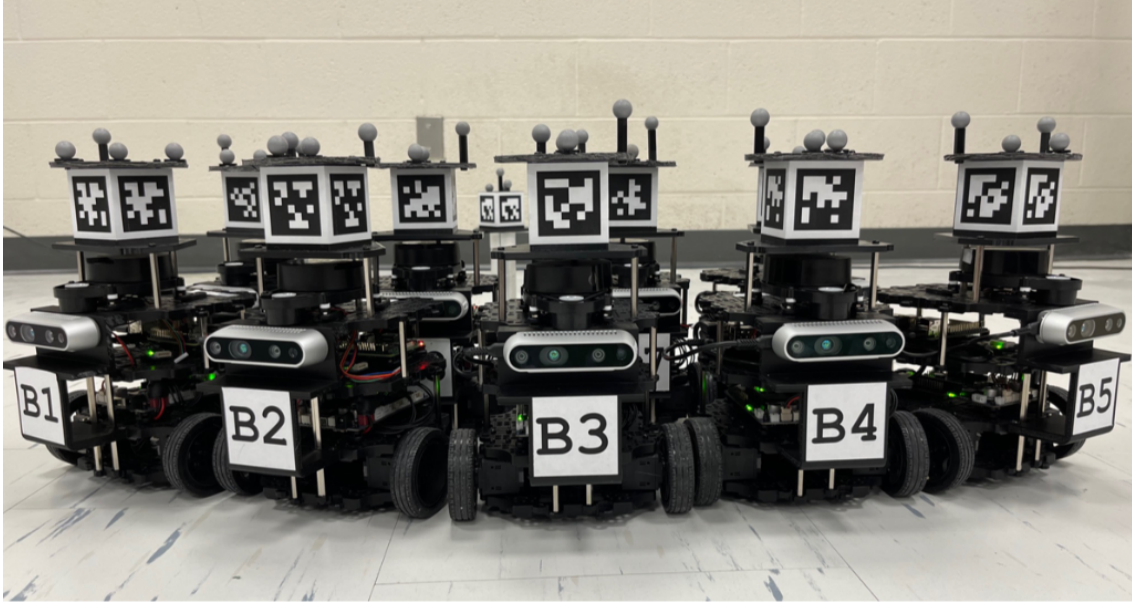
Figure 6.11: Image of a Turtlebot3 Burger used in the real robot experiment. It is fitted with AprilTag-labelled cubes, an Intel-Realsense D435i camera and Vicon markers. Vicon markers are only used to obtain the ground-truth trajectories, used for the evaluation. The depth image, laser scanner and IMU are not used in any of the experiments.
