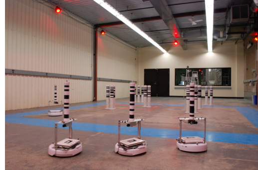
Figure 7.8: Robots used in the UTIAS MR.CLAM dataset. Each robot is equipped with a monocular camera and a barcode identifier. Images from [Leung et al., 2011].
