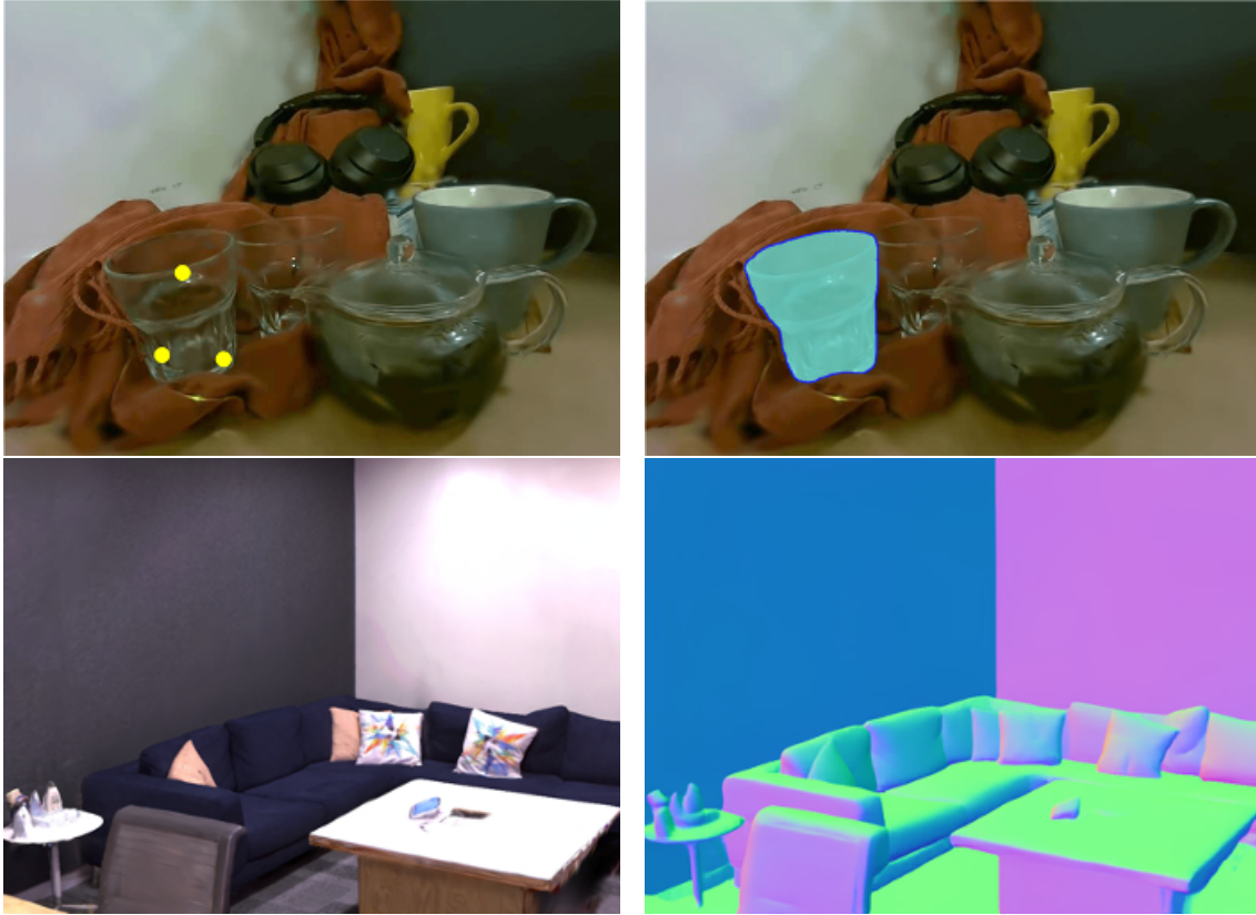
Figure 1.4: Running different off-the-shelf pre-trained models on a novel-view synthesis from Gaussian Splatting SLAM [Matsuki et al., 2024]. Top Row: Self-captured monocular reconstruction is segmented using Efficient SAM [Xiong et al., 2023], Bottom Row: Reconstruction of Replica RGB-D dataset is converted into a surface normal estimate using DSINE [Bae and Davison, 2024].
