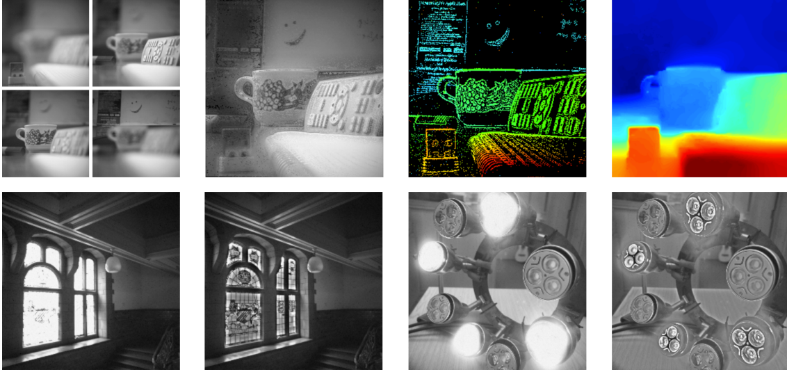
Figure 1.2: Example applications of SCAMP-5 FPSP. Top Row: Depth from focus [Martel et al., 2017]. Using a focus-tunable lens, images at different focuses are captured (left), and the sparse depth points (middle-right) are recovered by analysing the sharpness of each image using SCAMP-5. The right-most image is a post-processed, densified depth image. Bottom Row: HDR tone mapping [Martel et al., 2016], the pair of images shows images captured without HDR tone mapping (left) and with (right). Each pixel automatically determines the suitable integration time based on neighbouring pixel values by controlling the exposure time of individual pixels. Images are from [Martel et al., 2017, Martel et al., 2016].
