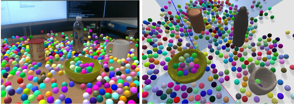
Figure 4.14: Few-shot augmented reality: Complete and watertight meshes can be obtained from few images due to the learned shape priors. This are then loaded into a physics engine to perform realistic augmented reality demonstrations.
