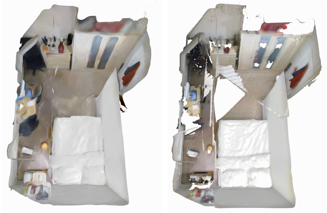
Figure 5.7: iMAP (left) manages to fill in unobserved regions which can be seen as holes in TSDF fusion (right).
