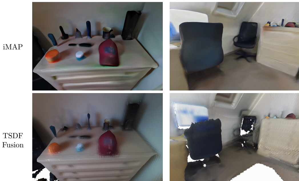
Figure 5.9: Comparative reconstruction results in various real scenes mapped with an Azure Kinect. White holes in the TDSF fusion results are plausibly filled in by iMAP, such as in black objects where a depth camera has missing data.
