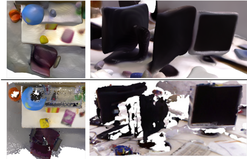
Figure 5.14: Hole filling capacity of iMAP (top) against BAD-SLAM (bottom).
