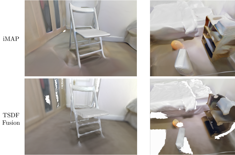
Figure 5.10: Comparative reconstruction results in various real scenes mapped with an Azure Kinect. iMAP can better represent thin structures and interpolate the back of objects.
