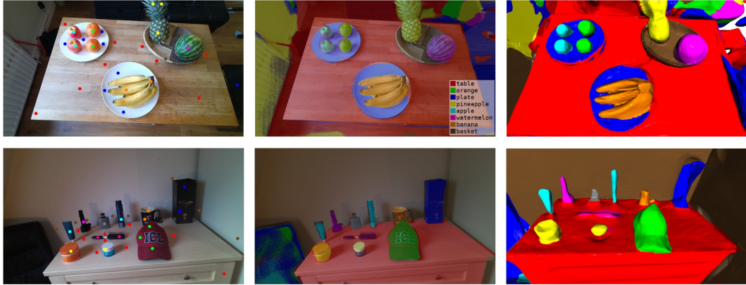
Figure 6.6: Precise segmentations can be obtained from just 1 or 2 interactive clicks per object. (Left: clicks; middle: dense labels rendered into a keyframe; right: full 3D mesh with labels.)
