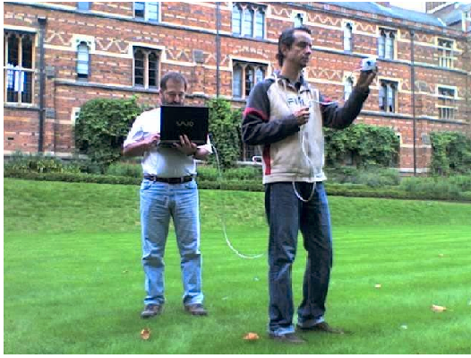
Fig. 1. Experimental setup: a hand-held camera, a firewire cable and a laptop.
