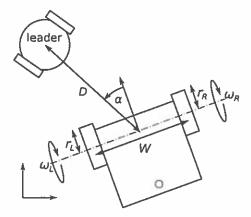
A low-level velocity controller is available which sets the rotation rates  $\omega_L$  and  $\omega_R$  of the left and right wheels respectively using the command SetMotorVelocity (port, omega), where port is left or right. The wheels have radii  $r_L$  and  $r_R$  and the distance between them is W.
