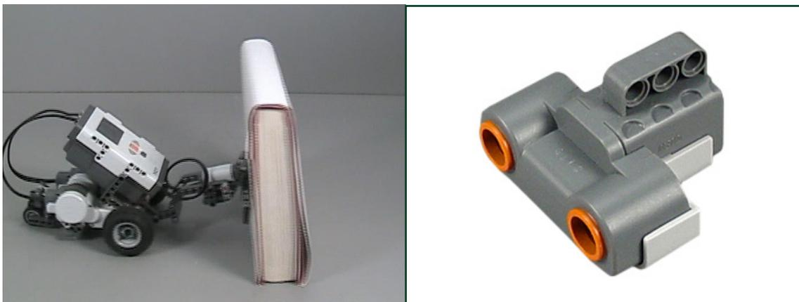
Above right is an Ultrasonic Sensor. Using the same physical principle that a bat or a submarine uses to find its way around, the Ultrasonic Sensor measures distances using sound. It then tells the robot how far away the nearest object in front of it is.
