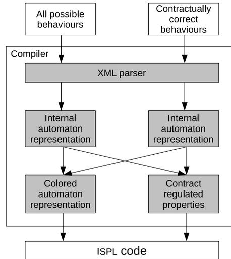
Figure 5. Internal architecture of the compiler
