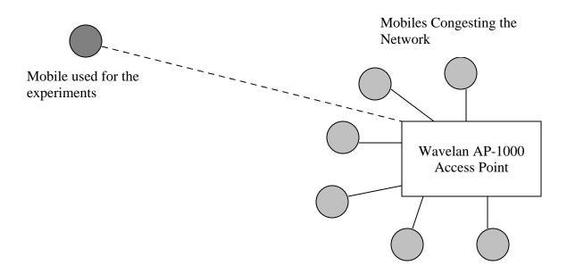
We used one of the mobile devices to perform the measurements while the other devices were congesting the network. To increase the signal to noise ratio, we moved the mobile device away from the access point. In the various runs of the experiment we kept changing the number of devices congesting the network and then using the other mobile to perform the measurements with varying signal to noise ratios.
