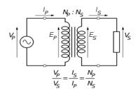
The primary objective in designing a current transformer is to ensure that the primary and secondary circuits are efficiently coupled, this will reduce any interferences so that the secondary current bears an accurate relationship to the primary current.
