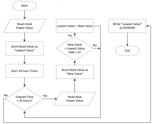
The following flowchart details the process of this self-calibration:
