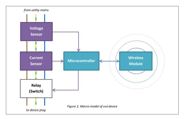
The microcontroller reads the values from the voltage and current sensor – these are both simplex data communication lines. Based on these reading and commands from the central hub, another simplex line can be used to send control instructions to the relay. Note that the microcontroller interfaces with the wireless module in a half-duplex mode – at any given instant, communication can only occur in one direction, even though it is a bidirectional communication link.
