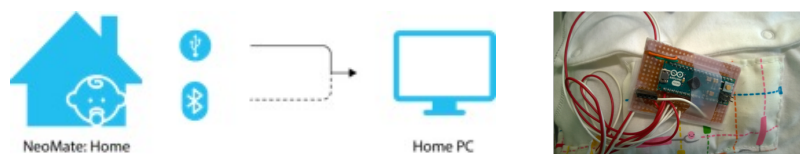
Figure 3: (Left) NeoMate: Home communications; (Right) Prototype board with Arduino Micro, hardwired sensors and female header pins to attach HC06 Bluetooth module
