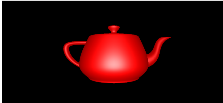
Figure 3: Result for Task 3b: Blinn-Phong shading at identity view matrix with camera z location at -37 and a light intensity of 500.0. ambient = (0.5,0,0,1), diffuse = (1,0,0,1), specular = (1,1,1,1), shininess=10
