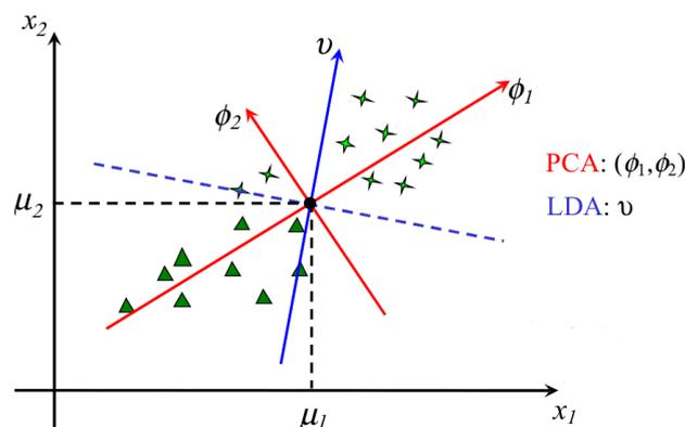
The above figure illustrates the difference between PCA and LDA. In PCA we take the data as a whole and do not consider any division into classes. The axes are optimal for representing the data as they indicate where the maximum variation actually lies. The LDA axis is optimal for distinguishing between the different classes. In
