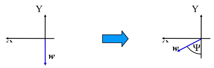
So the last two rotations can orient *w* in any direction in the 3D space.
