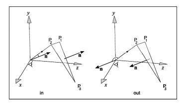
Q2. Using Lambert's cosine law, the brightest point in the triangle will be where the angle between the surface normal and the light direction is closest to zero.
