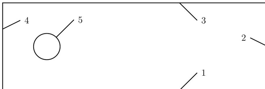
Figure 8.7: The boundary facet labelling used for our test problem. Labels 1 – 4 are assigned automatically by the mesh generator and the cylinder was declared to have label 5.
