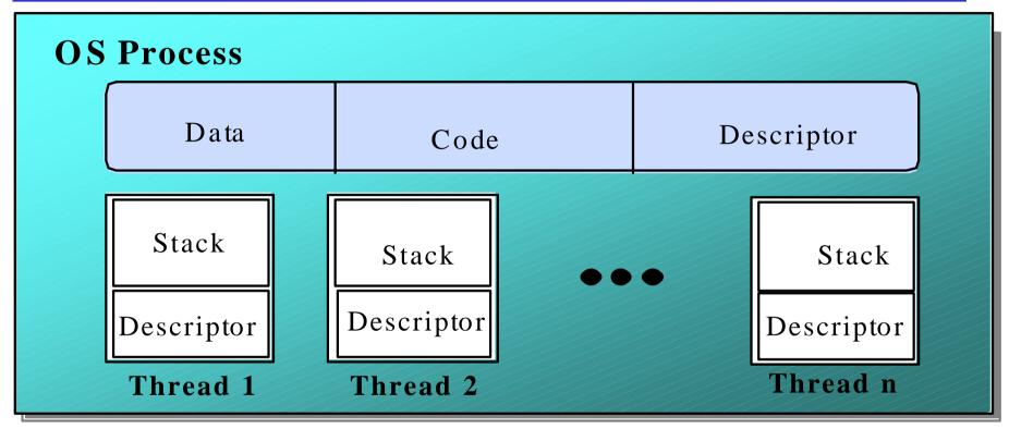
A (heavyweight) process in an operating system is represented by its code, data and the state of the machine registers, given in a descriptor. In order to support multiple (lightweight) **threads of control**, it has multiple stacks, one for each thread.
