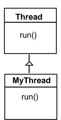
The Thread class executes instructions from its method run(). The actual code executed depends on the implementation provided for run() in a derived class.
