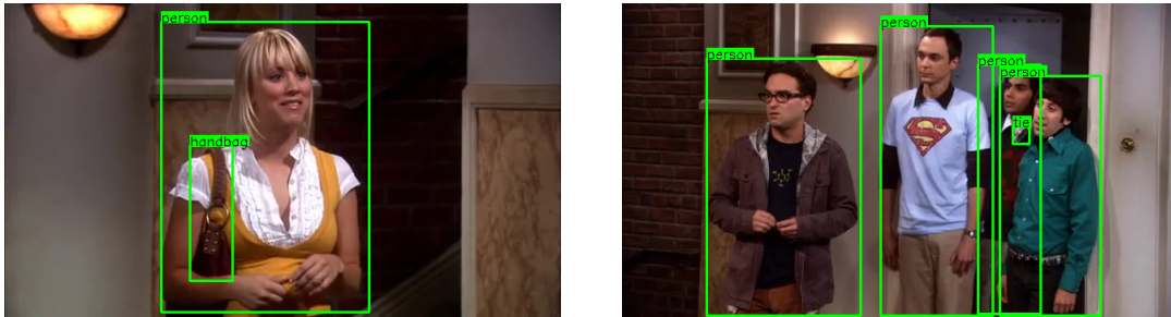
Figure 4.4: A demonstration of object detection with torchvision 's pre-trained Faster R-CNN with ResNet-50-PFN backbone.
