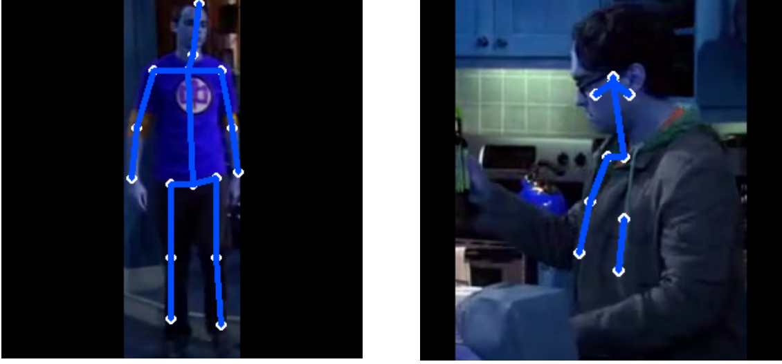
Figure 4.8: Human pose estimation on TVQA+ data. The blue sticks represent the limbs and body chunk, while the circles represent the joints.
