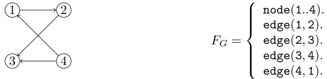
Figure 1: An example of a Hamiltonian Graph G and its corresponding representation in ASP, F_G .
