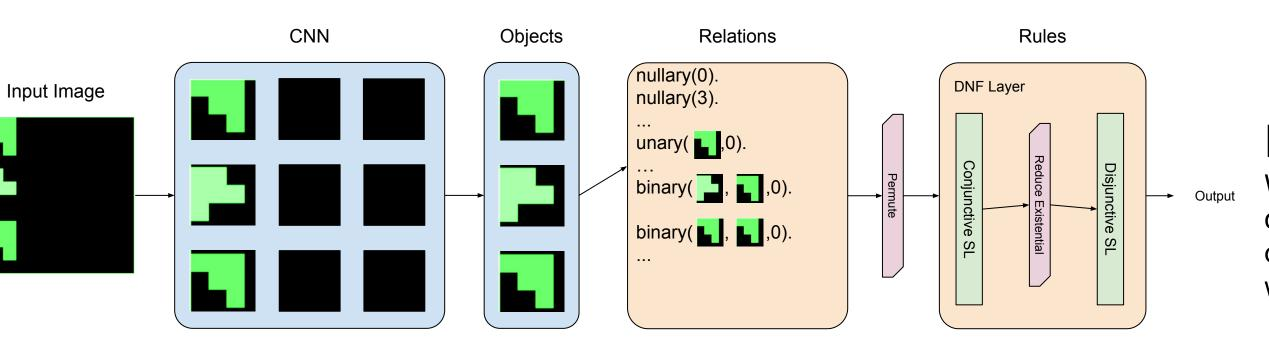
For the full neuro-symbolic model, we combine the DNF layer with an upstream Convolutional Neural Network, object selection and relational layers. The entire model is **end-to-end differentiable** and the object representations, their relations and rules are learnt together. For symbolic tasks we just use the DNF layer as a standalone model.
