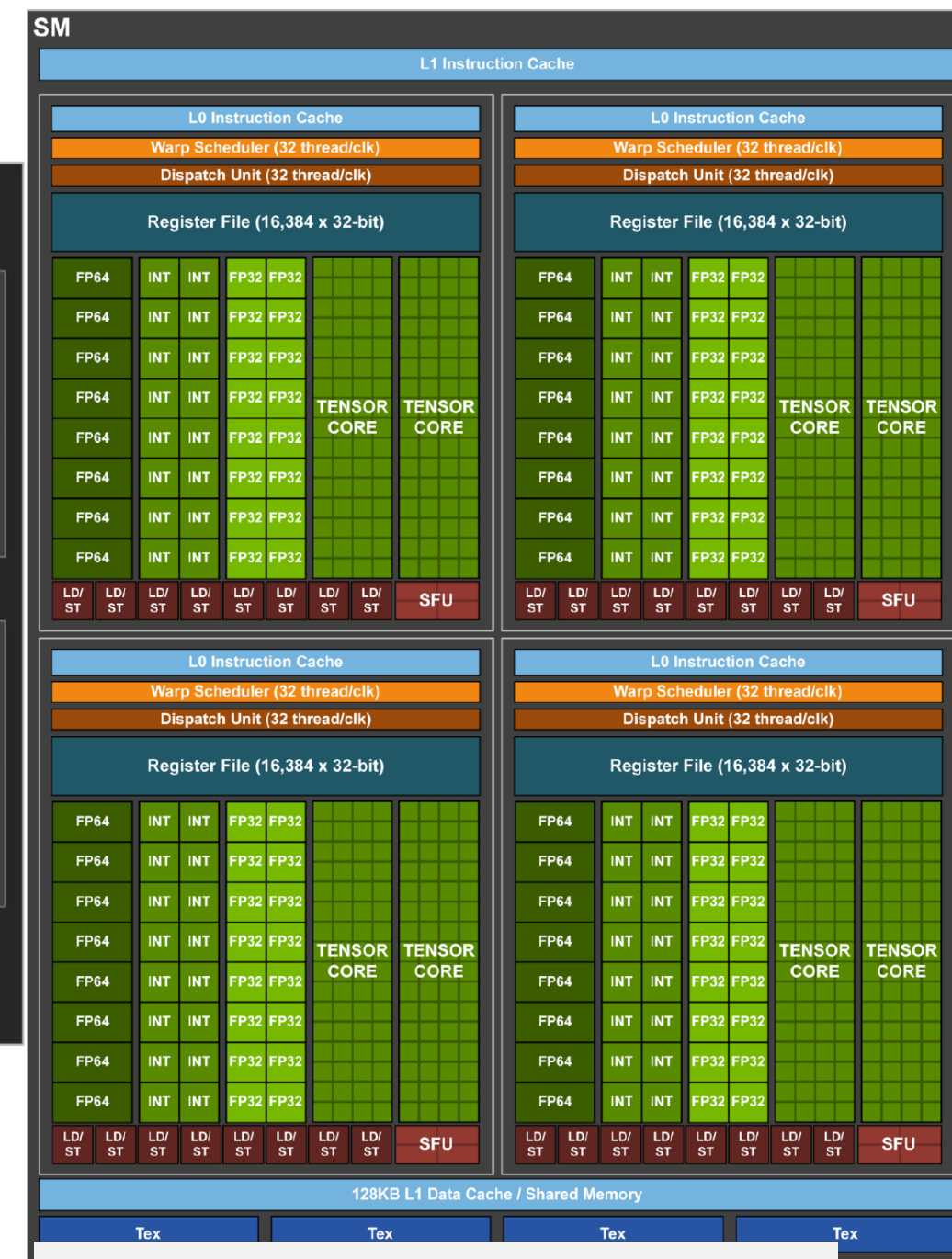
GV100's SM includes 8 tensor cores
