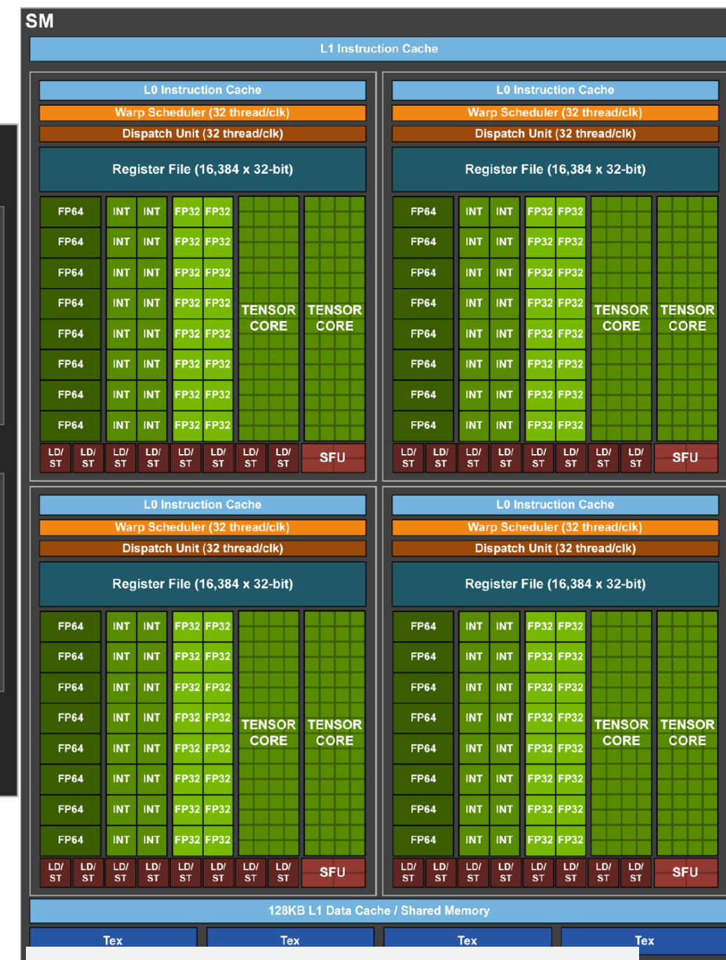
GV100's SM includes 8 tensor cores
