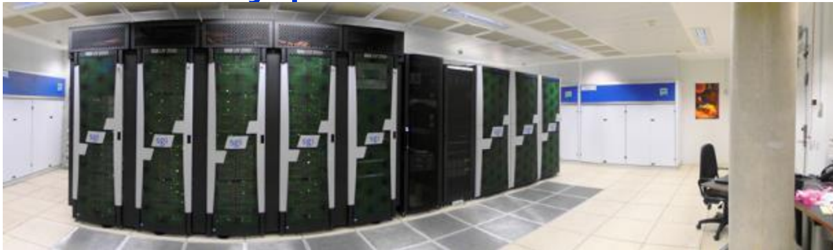
COSMOS: UK National Cosmology Supercomputer. SGI Altix UV 2000 with 1536 cores and 12.2TB RAM, globally accessible (delivered 2012)
