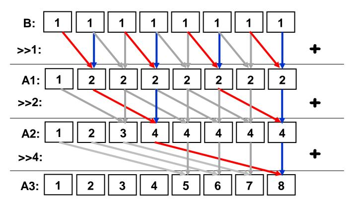
We can see that the last element is computed with a reduction tree
