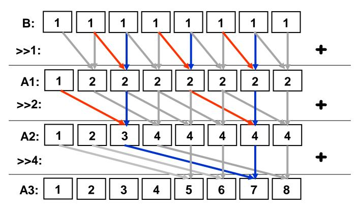
All the elements are computed by reduction trees of depth log(N) – for example element 7
