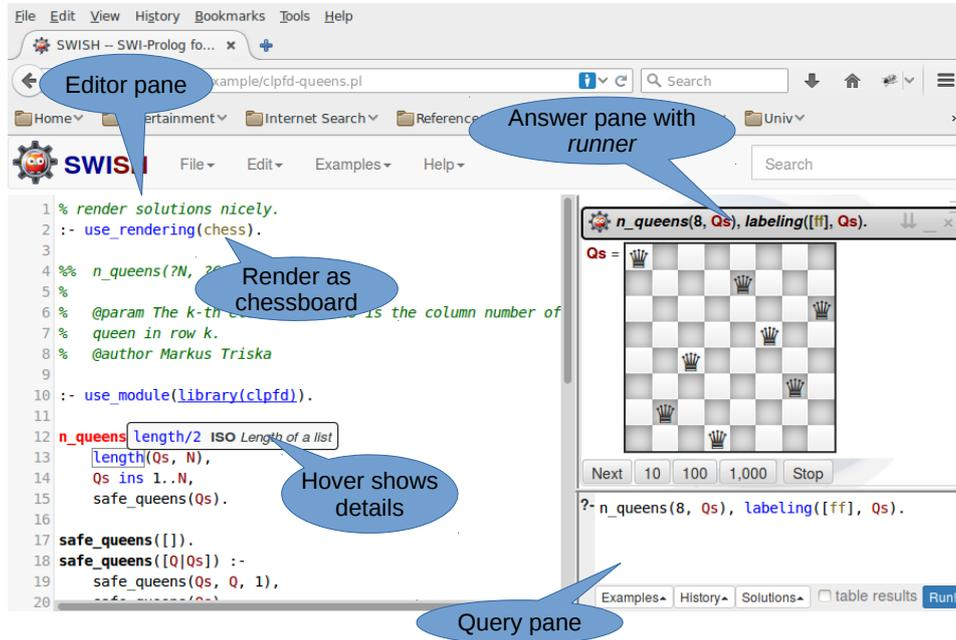
Fig. 1. Screenshot of SWISH in ‘IDE’ mode. The left pane holds the source code editor, while the top-right pane holds a query *runner* that exploits the current selected answer *renderer* and buttons for continuing after the first answer. The bottom-right pane holds the query editor with access to example queries stored in the source, query history, solution modifiers, result presentation and a Run! button to start the query.
