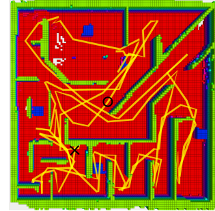
Fig. 6. Top-down view of a map of the maze environment created by our algorithm. Voxels are coloured based on their height, with red indicating floor voxels and green voxels near the cropped roof. The MAV's starting position is marked by a black circle, its path by a yellow line and its final position by a black cross.
