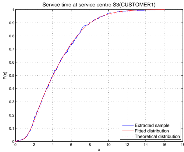
Figure 5.26: Comparing the best-fit hyper-Erlang distribution with extracted samples and theoretical distribution for service time for CUSTOMER1 at service centre S3 in case study 3
