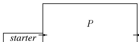
Figure 2 The overall layout for a user program P with the starter block. The arrows indicate the location of the req and ack signals for P .
