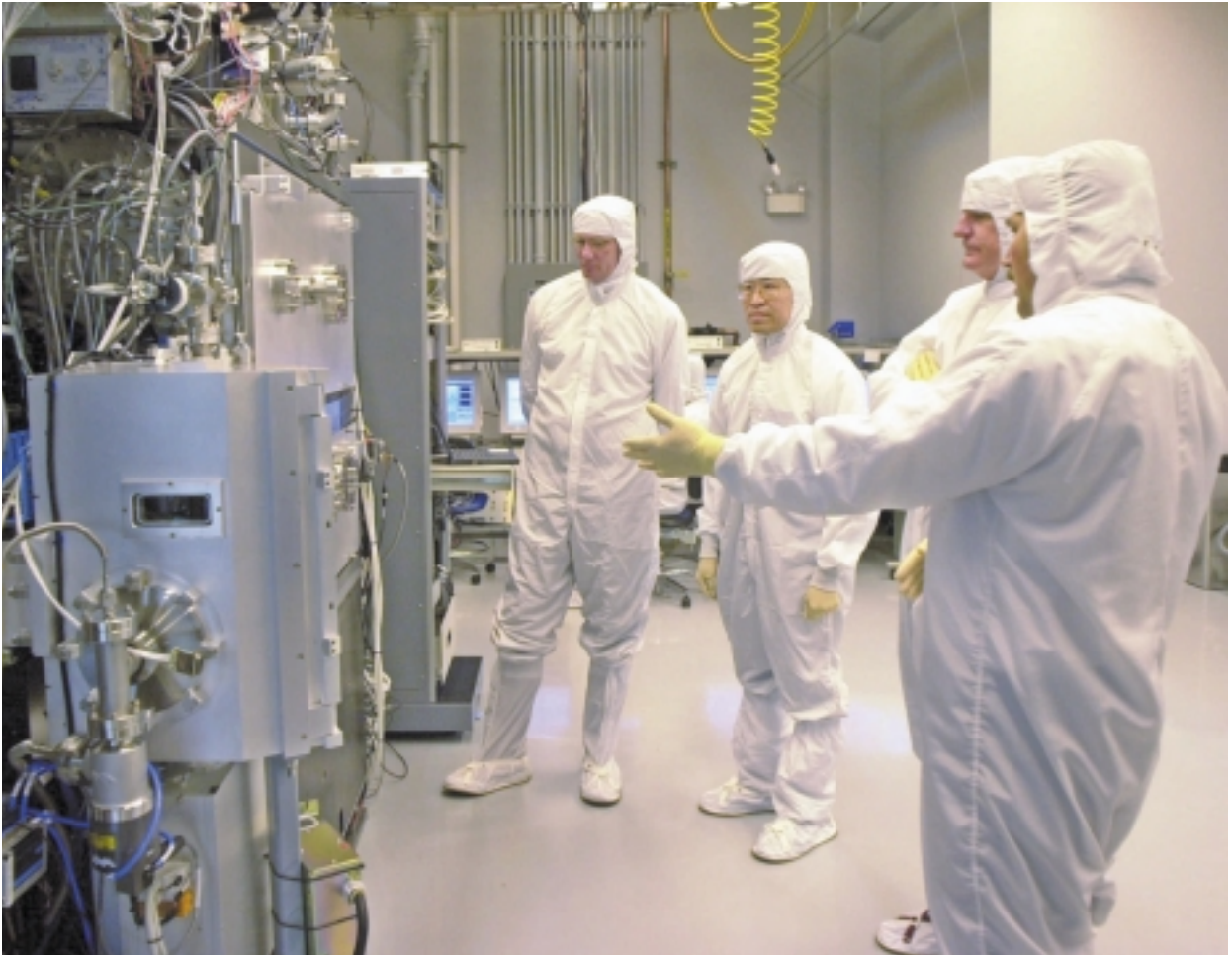
Microprocessors hundreds of times as powerful as today's should emerge from chip-making equipment using extreme ultraviolet radiation. Sandia National Laboratories unveiled such equipment a year ago [above].
