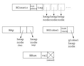
Figure 5. Heap Node Structures
