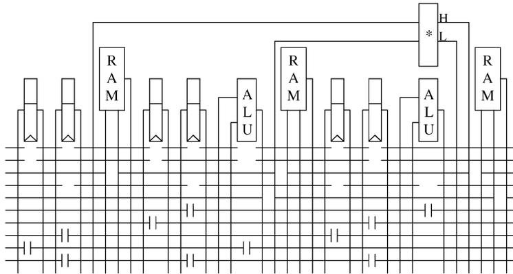
**Fig. 7.** One cell in the RaPiD-I reconfigurable architecture [Ebeling et al. 1996]. The registers, RAM, ALUs, and multiplier all operate on 16-bit values. The multiplier outputs a 32-bit result, split into the high 16 bits and the low 16 bits. All routing lines shown are 16-bit wide busses. The short parallel lines on the busses represent configurable bus connectors.
