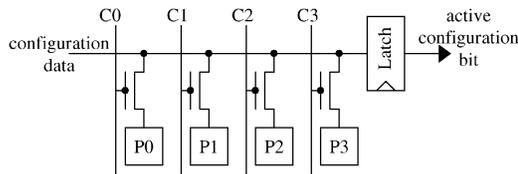
**Fig. 15.** A four-bit multicontexted programming bit [Trimberger et al. 1997a]. P0-P3 are the stored programming bits, while C0-C3 are the chip-wide control lines that select the context to program or activate.
