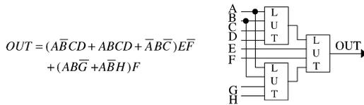
**Fig. 12.** A wide function implemented with multiple LUTs.
