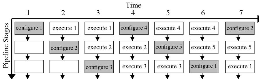
**Fig. 16.** A timeline of the configuration and reconfiguration of pipeline stages on a pipeline reconfigurable FPGA. This example shows three physical pipeline stages implementing five virtual pipeline stages [Cadambi et al. 1998].
