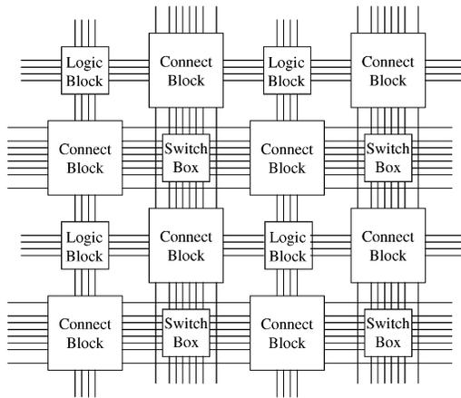
**Fig. 5.** A generic island-style FPGA routing architecture.
