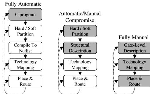
**Fig. 11.** Three possible design flows for algorithm implementation on a reconfigurable system. Grey stages indicate manual effort on the part of the designer, while white stages are done automatically. The dotted lines represent paths to improve the resulting circuit. It should be noted that the middle design cycle is only one of the possible compromises between automatic and manual design.
