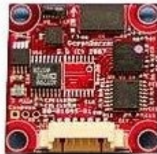
Fig.13. Ocean Server OS5000 3 Dimensional Compass
